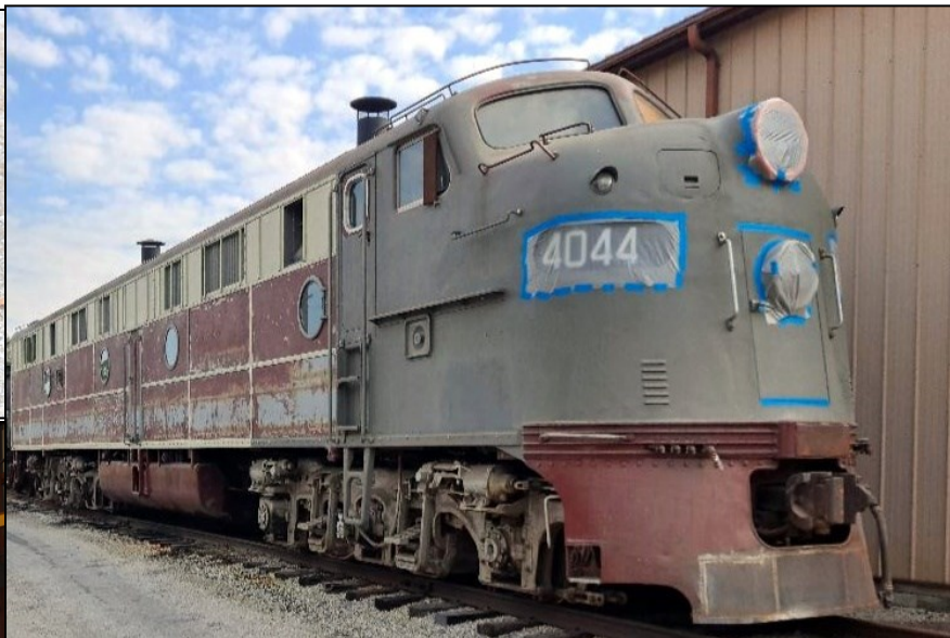
The E-8 Locomotive no. 4044 is coming to life with the installation of a set of batteries, nearing the completion of restoration to operation. The locomotive is being masked in preparation for painting in the IC colors.
