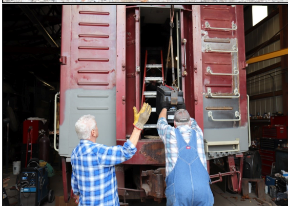
The E-8 Locomotive no. 4044 is coming to life with the installation of a set of batteries, nearing the completion of restoration to operation. The locomotive is being masked in preparation for painting in the IC colors.
