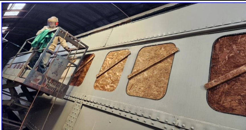
The E-8 Locomotive no. 4044 is coming to life with the installation of a set of batteries, nearing the completion of restoration to operation. The locomotive is being masked in preparation for painting in the IC colors.
