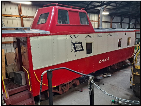
Wabash 2824 is undergoing interior restoration for static display with a display cabinet beneath the cupola seats and electric lights.
