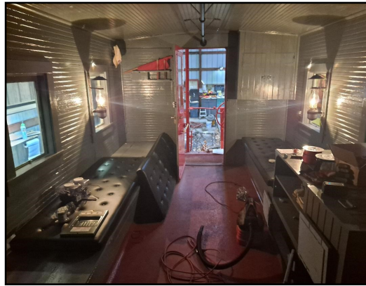
Wabash 2824 is undergoing interior restoration for static display with a display cabinet beneath the cupola seats and electric lights.
