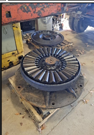
Above Left and Lower Left: Side panels being applied. Above: Bearings for the Turntable base. Right: Members are working on the shutters of RS-3 Alco.
