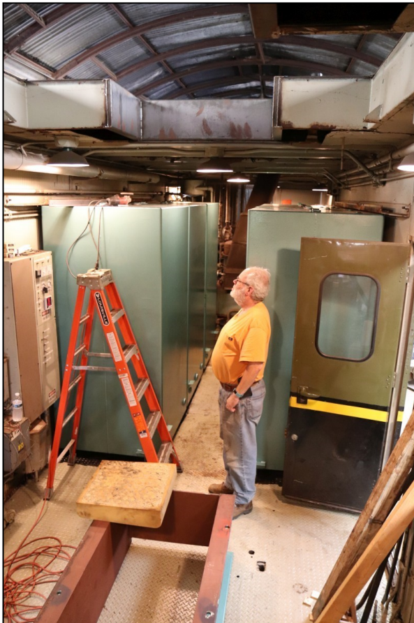
Above Left: Eric Schafer looking at work required to anchor the tops of the water tanks to the car sides. Lower foreground shows the base for the new genset in place. Above Right: New genset installed in CN 15421, shortly before applying the roof hatch.
