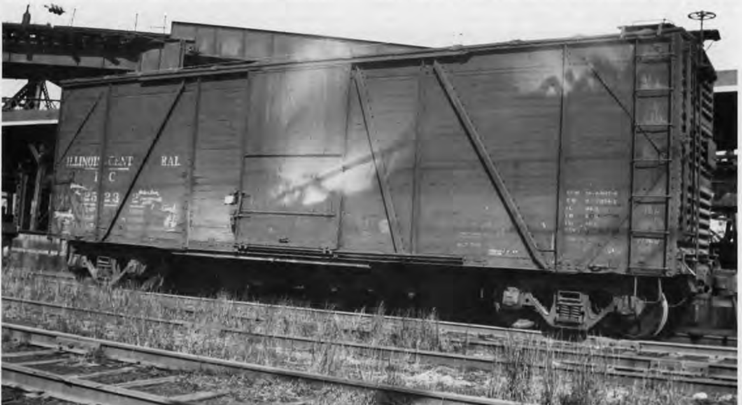
Illinois Central boxcar #25232 shown in service in New York in 1949. Note the three panel car end. Photo Collection of Jerry Carson
