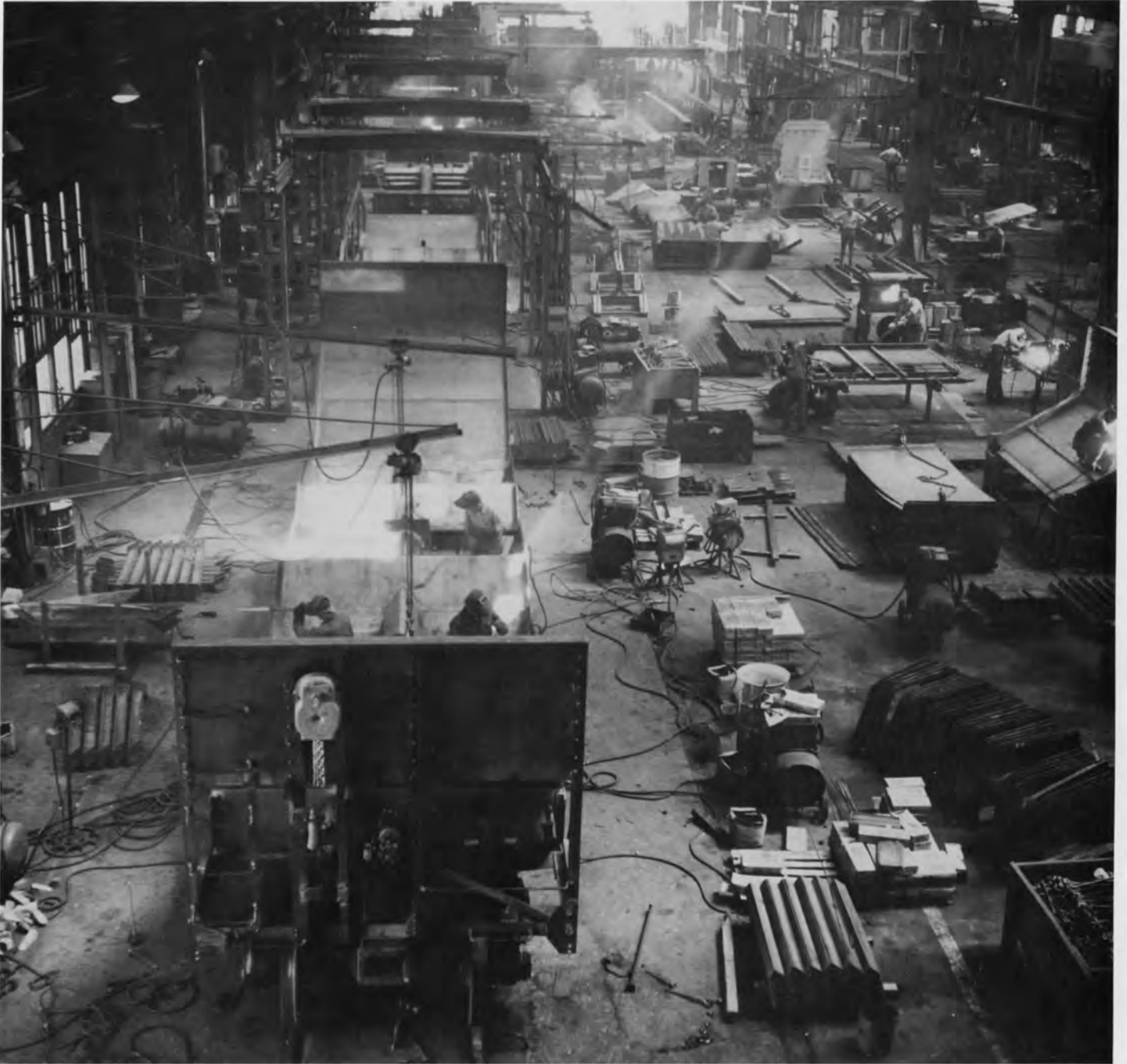
The photo above is looking back down the assembly line on track 8 again as a car has taken shape in the foreground. The floor sheets and ends have been installed. The end floor sheeting jig is seen at the right.
