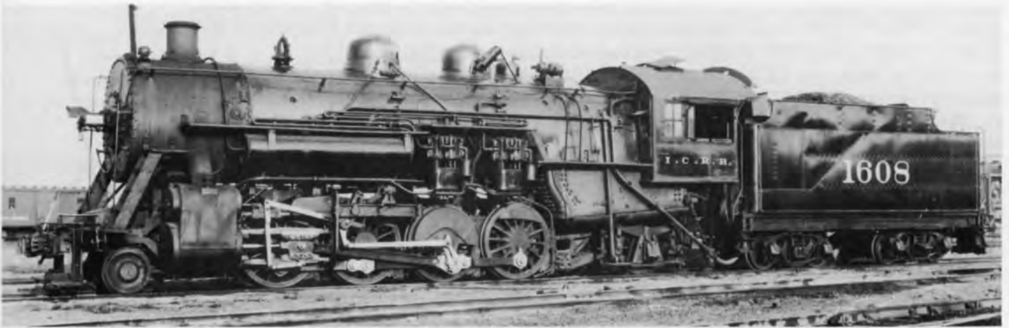
One of the first group of Mikados received from Baldwin in 1911 was #1608. This "Mike" became an 0-8-2 during rebuilding in 1942 and was renumbered #3682. It remained in service for the IC until 1953. photo from the collection of Mike Schafer.
