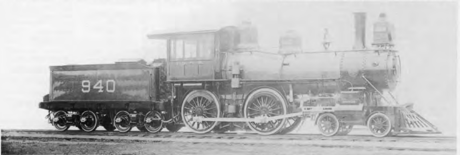
#940. From the same lot as ISRR #91-95 (Brooks 1894) #940 presents a classic late nineteenth century look in this builders photo. It undoubtedly ranged to and from between Effingham and Indianapolis with a two to four car consist. This engine became #1940 and then #4940 and was retired in 1928. Alco Historic Photo, Author's Collection.
