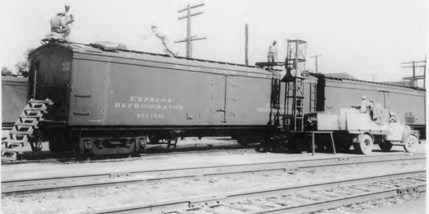
Pre-cooling of refrigerator cars was hard work in the days before mechanical reefers. Here, with the help of a special lift truck, an REA reefer is loaded with ice at Hammond, Louisiana in 1953. The next car is a PFE reefer. C. W. Witbeck photo.
