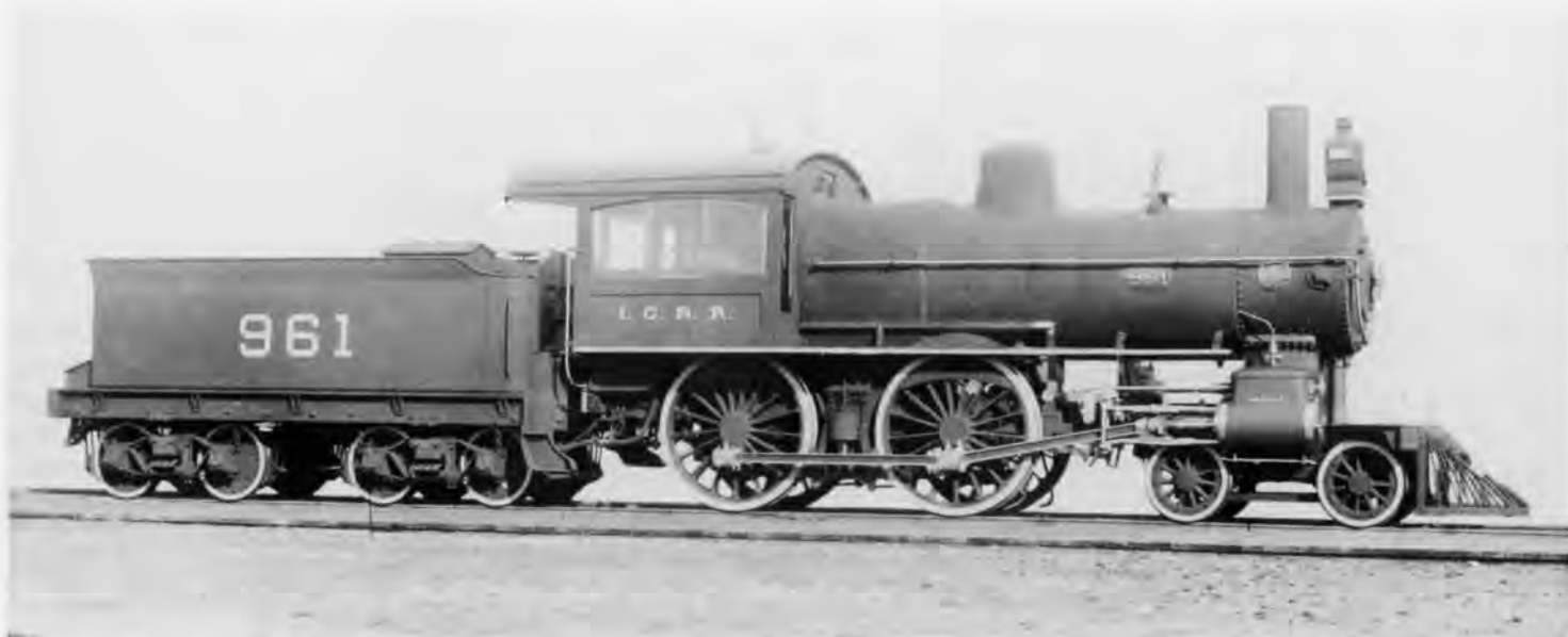
#961. This trim "English-American" was assigned and served Indianapolis through the teens. Brooks-built in 1896, the clean, sleek, uncluttered design, with the engine number on the boiler below the bell was definitely English in appearance. The nine engines in this class must have been run to death, for they were all retired in 1926. Alco Historic Photo, Author's Collection.
