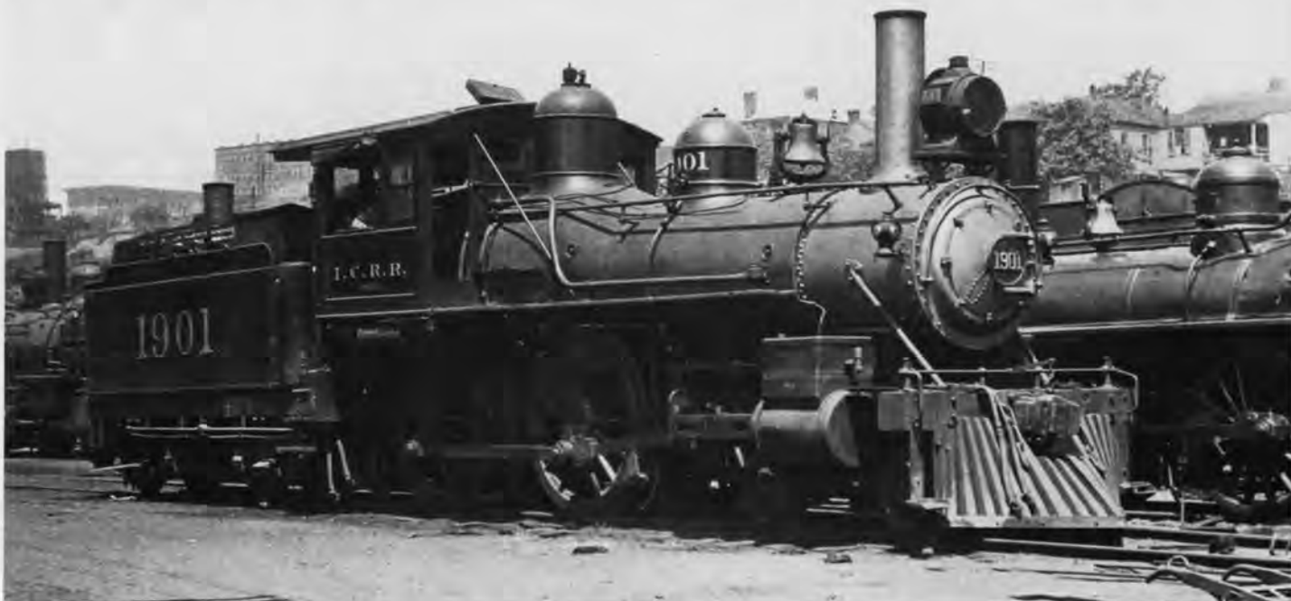
IC #1901 was built by IC shops in 1888 with 18"x 24" cyl. & 69" dr.. Originally #161, #901, #1901, and later #4901. retired in 1927. Jerry Carson Collection
