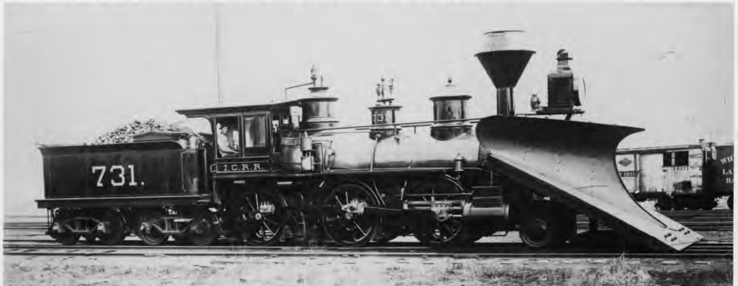
#731 2-6-0 Engine Snow Plow started life as #6 on the IC roster, was renumbered #466, then #731 in 1890. After 1903 she carried #1731 until 1915 when reassigned #2731 which lasted until scrapping in 1916. Built by IC shops in 1880. 18"x 24" cyl., 56 1/2" dr. The IC car in the background is one of the 28' 6" fruit cars of 14 ton capacity. The photo dates from 1890's C.W. Witbeck photo Tom Grant Collection
