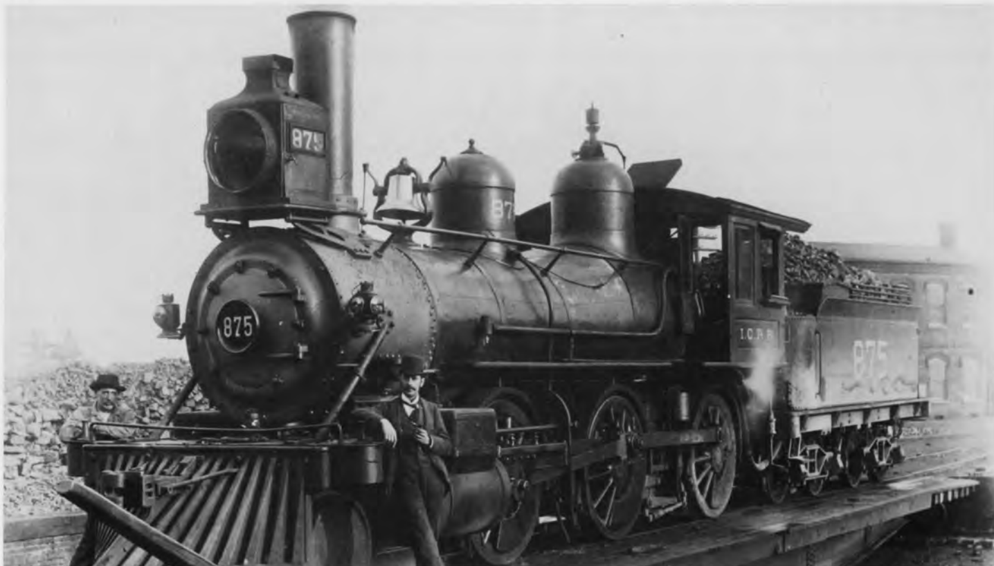
A former Chesapeake & Ohio Southwestern Loco, IC #875 is shown at Paducah Ky. in 1898 in this R.A. Beck photo. The #875 also wore #419, #507, & #1875 while on the IC roster. Built by Hinckley in 1888, she was retired in 1914. 18"x 24" cyl., 56 1/2" dr. photo Jerry Carson Collection
