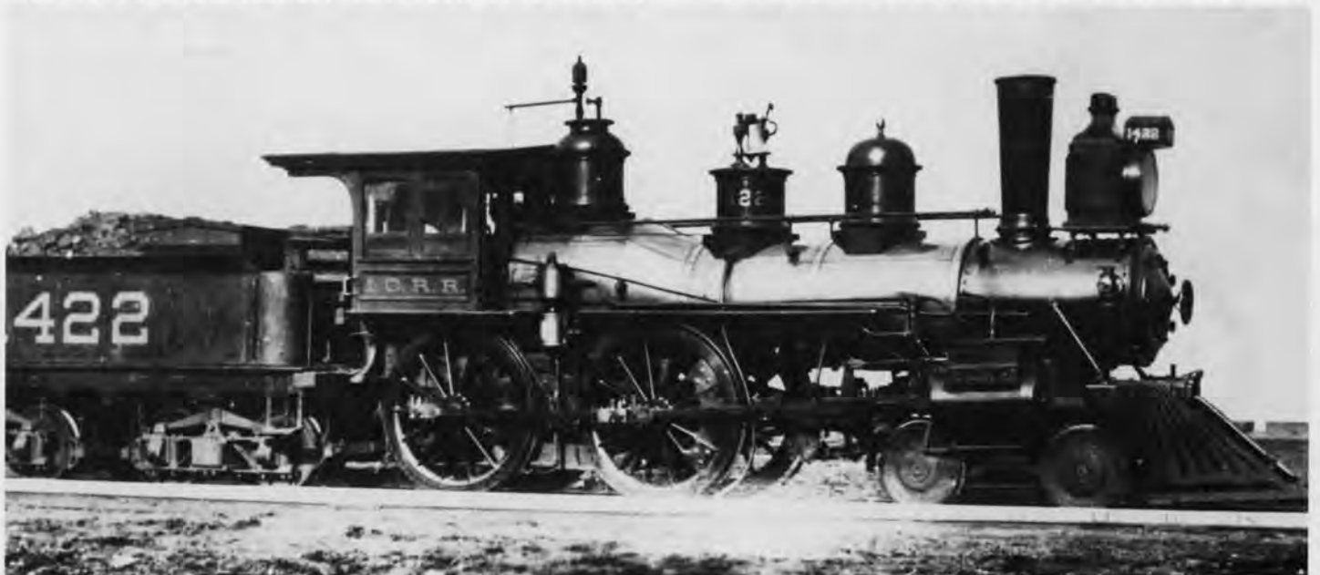
Built by Rogers, originally as IC #50 in 1854, the #1422 was renumbered in 1890 and dropped from the roster by 1896. 14 1/2"x 22" cyl., 60" dr.
