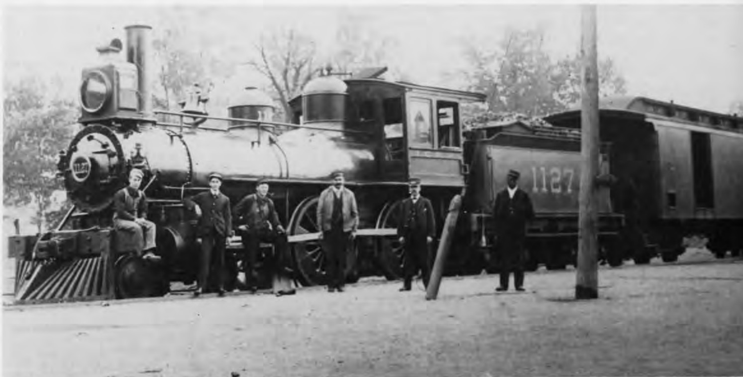
#1127 shown at Martin Tennessee about 1904. This engine was assigned to Water Valley Miss. in the 1890's. Built by IC shops in 1871 with 16"x 24" cyl. and 60" dr., retired in 1915. The engine shows on a Dec. 22, 1893 train register on train #1 with Casey Jones as engineer. Bruce Gurner Collection
