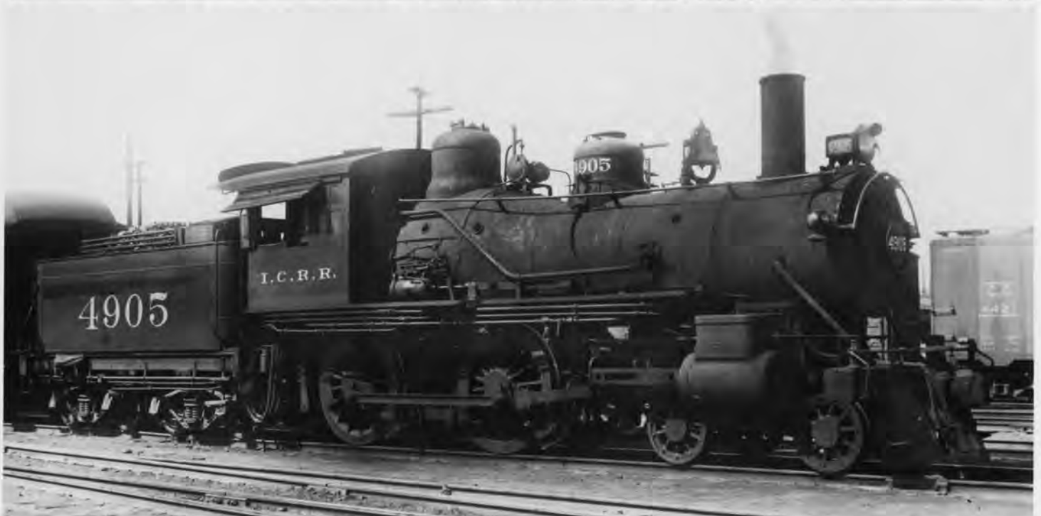
This photo of #4905 shows an early 4-4-0 after rebuilding and modernizing. Built by Brooks in 1890 with 18"x 24" cyl. & 64" dr.. This 4-4-0 remained on the roster until 1940. Previous numbers were #905, & 1905.
