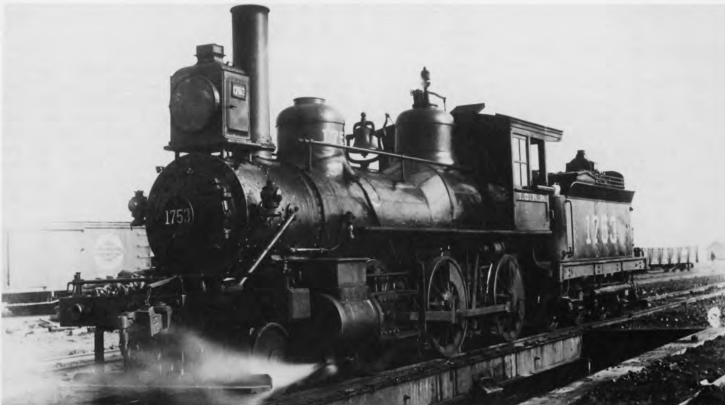
2-6-0 #1753 shown here at Amboy Ill. in 1904, was built by the IC shops in 1881 and originally numbered #218, then #753, and renumbered #1753 in 1903. 18"x24" cyl., 56 1/2" dr. photo Jerry Carson Collection
