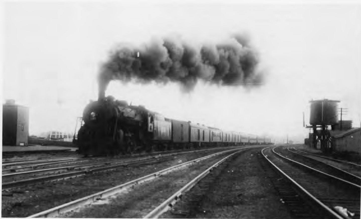
Pacific #1156 and train at an unknown location, possibly Jackson Mississippi with a dry insulated express refrigerator (no roof hatches), a 64' mail storage car, probably 600 series, a 64' mail-baggage car (297-300 series), two more 64' baggage cars, and a string of coaches. Photo from the collection of Ted Richardson.
