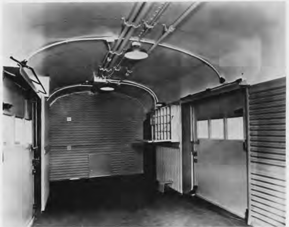
Interior of the baggage compartment looking forward toward the RPO compartment. Note the small access door to the RPO. This was to thwart would-be robbers. Collection of Robert E. McMillan.
